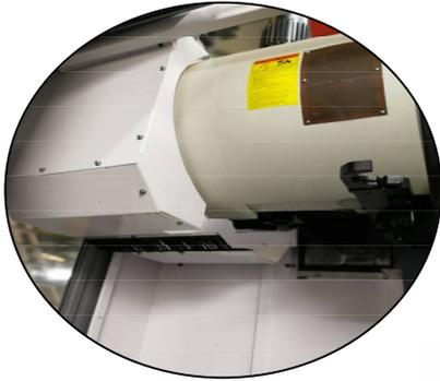
Shoulder carrying Taiwan brand tool magazine with cover to ensure Z axis geometric precision and durability
