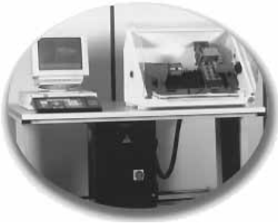
Fig. 25 Novaturn A compact 2 axis CNC bench turning center suitable for all levels of education and technical training. The Novaturn is controlled via a standard keyboard or Desk-Top Tutor connected to a PC. (Denford Inc.)
